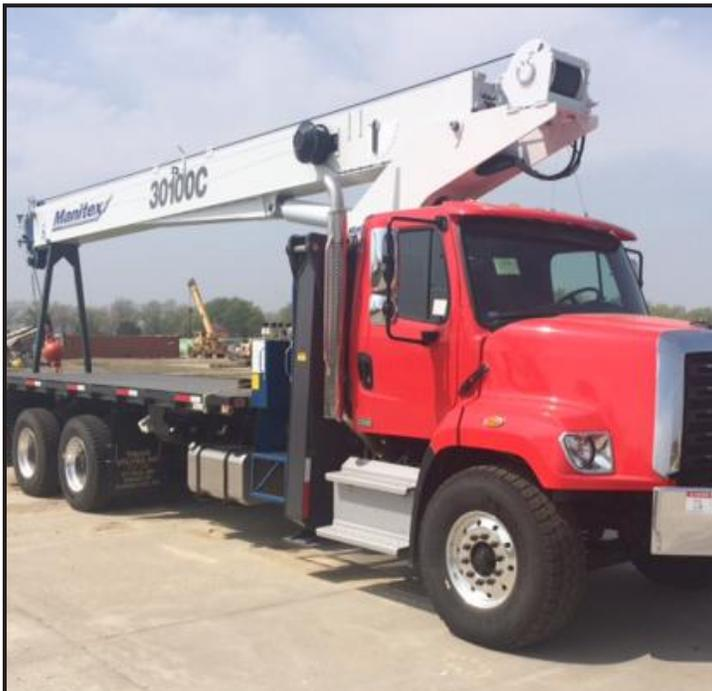
The Sunflower Division's new 2015 30 ton Manitex Crane shown here mounted on a 2015 Freightliner Chassis.
